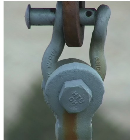
RIGHT: This image, taken using Klickitat PUD's drone, shows attachment failure on a high voltage transmission conductor. This issue was easily identified using drone inspection methods.
