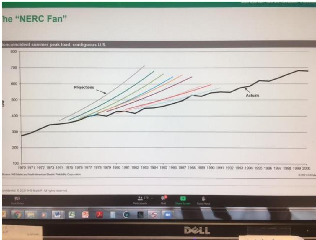
This chart shows the actual DEMAND curve in that same time period and also shows the projected demand. Each line is the projection for that year and shows how the projections were flattening out.
